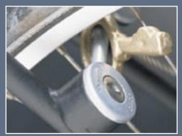
The bicycle key is inserted into the existing lock on the bicycle, thereby dispensing with the need to carry an extra wire lock for the bicycle.
