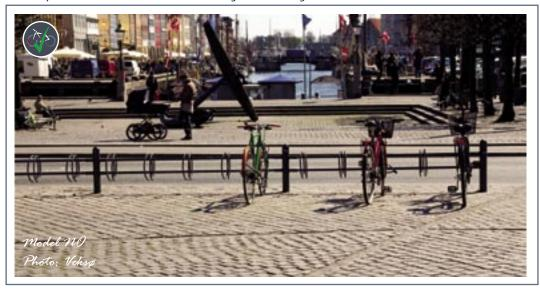
The butterfly rack must be wedge-shaped; otherwise it will not fit all tyre widths.
