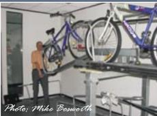
Two-tier parking with a ramp to ease lifting is a good solution for larger facilities. This stand is from Orion Bausysteme (Germany).
