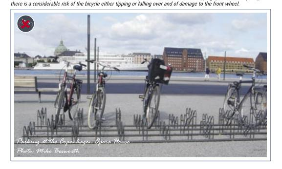
Horizontal butterfly racks are not recommended under any circumstances. This stand type grips the wheel poorly, and
