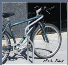
Vertical butterfly rack with supplementary support and possibility of securing bicycle – model KL80 from Veksø.
