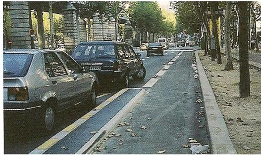
Figure 16 – Intersection without traffic lights - the physically separated cycling path becomes a cycling lane before the intersection and on street parking is not allowed 20m before the intersection (Source: Recommendations pour les aménagements cyclables, CERTU, 2008)
