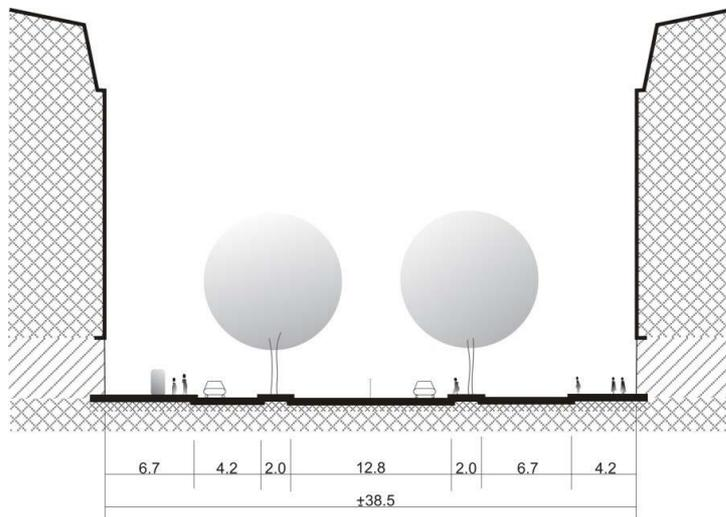
Figure 52 - Cross section Avenue Montaigne
