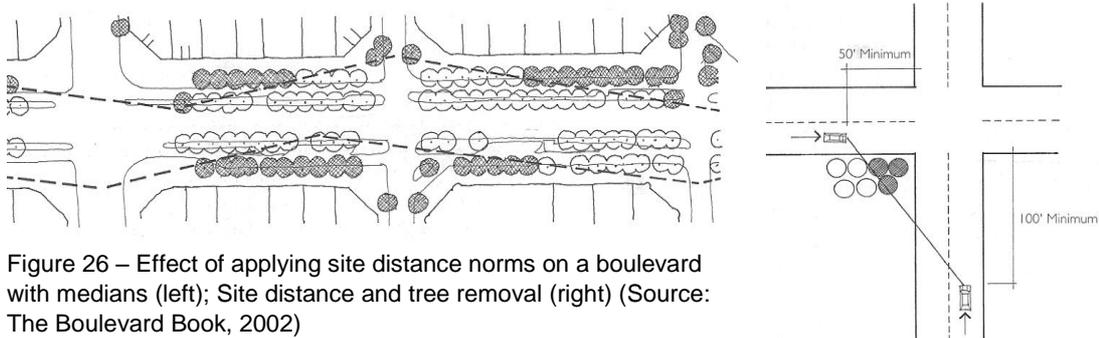
Figure 26 – Effect of applying site distance norms on a boulevard with medians (left); Site distance and tree removal (right) (Source: The Boulevard Book, 2002)
