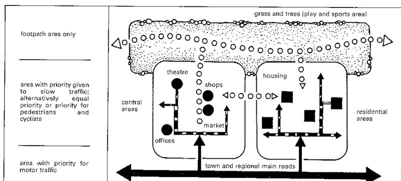
Figure 18 – Diagram representing the principle of cell and artery and the separation between pedestrian network and major traffic arterials (Source: Neufert, Third Edition, 2000)
