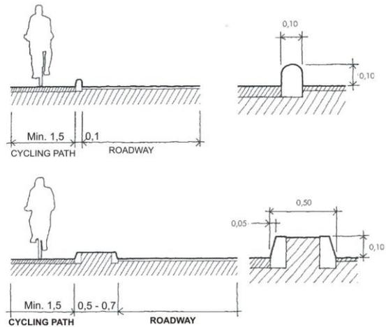
Figure 13 – Cycling paths physically separated from the roadway – Top: on the roadway by a raised curb; Bottom: between the roadway and the sidewalk (Sources: Manual de las vías ciclistas de Gipuzkoa, Diputación Foral de Gipuzkoa, 2006 and www.eltis.org)
