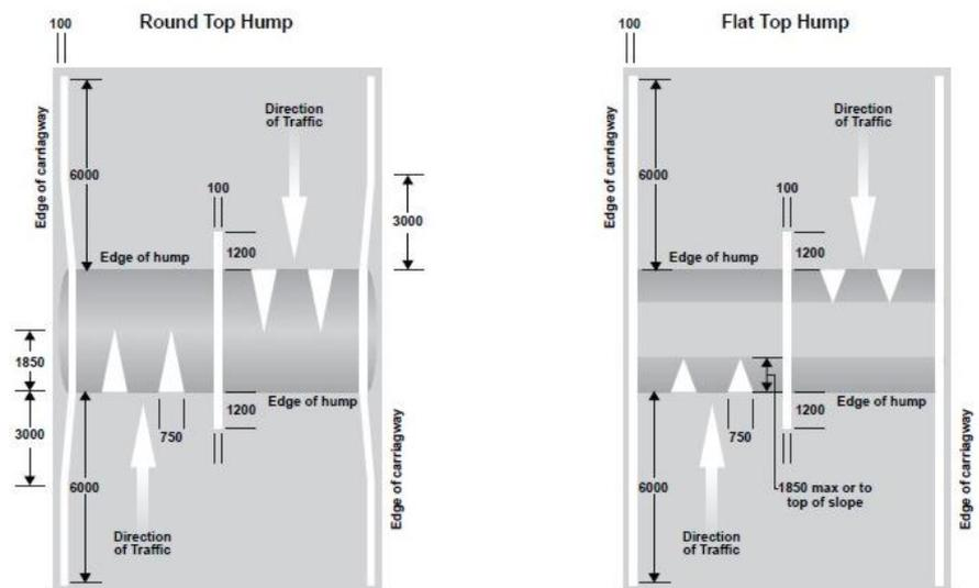
Figure 28 – Speed hump technical details and photo (Sources: Local Transport Note1/07- Traffic calming, Departament for Transport, March 2007 and O. Stepan)
