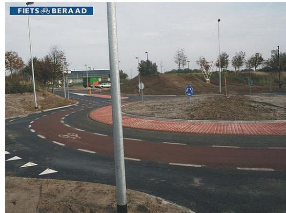
A cycle lane marked in the middle of the roundabout lane
