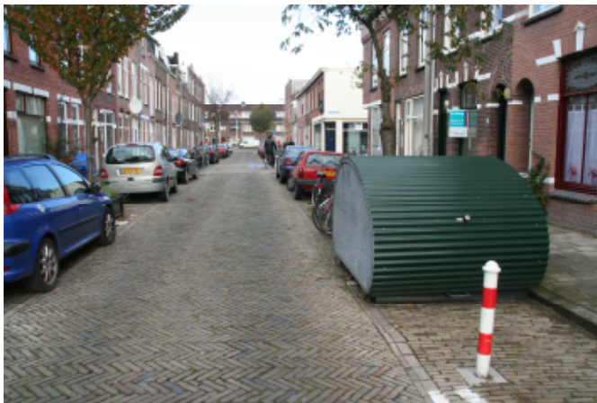
A cycle drum on the parking lane in a residential street, with a bollard protecting access. Utrecht, NL 2
