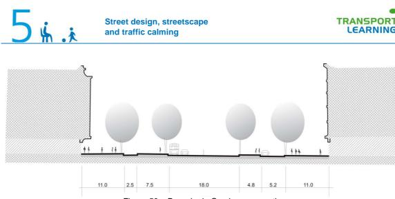
Figure 58 – Passeig de Gracia cross section
