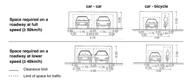
Figure 6 – Space required by cars on a roadway depending on their speed (Source: Neufert, Third edition, 2000)
