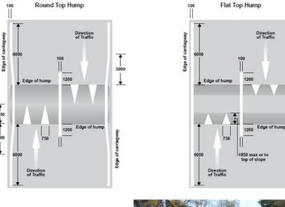
Figure 28 – Speed hump technical details and photo (Sources: Local Transport Note1/07- Traffic calming, Departalent for Transport, March 2007 and O. Stepan)
