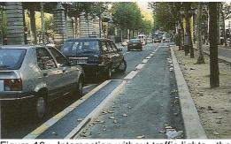
Figure 16 – Intersection without traffic lights - the physically separated cycling path becomes a cycling lane before the intersection and on street parking is not allowed 20m before the intersection (Source: Recommandations pour les aménagements cyclables, CERTU, 2008)
