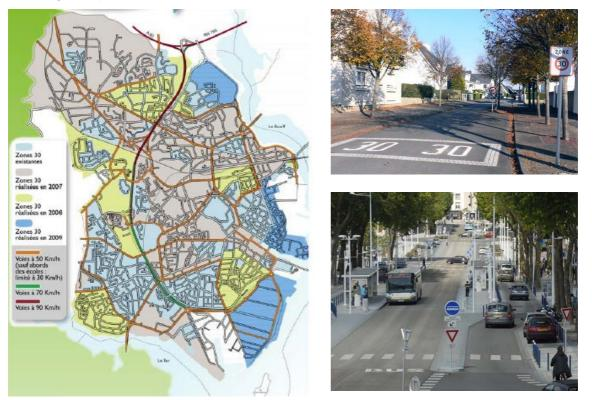
Figure 34 - Plan for implementing 30 zones in Lorient, France - The implementation of 30 zones all over the city was made step by step based on a coherent classification of the street network (left); The residential 30 zone - 30 zones are present in almost all residential areas in the city (right-up); Avenue Anatole France in Lorient – the 30 zone allows an easy cohabitation between all transport modes (Source: *Zones à circulation apaisée*, Fiche 1, CERTU, 2008)
