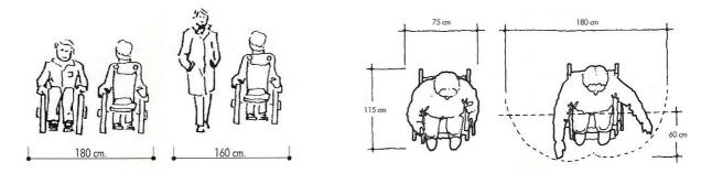
Figure 2 – Passing space (left) and Turning space (right) – minimum dimensions required by wheelchair users on footway (Source: Calmar el trafico – Pasos para una nueva cultura de la movilidad urbana, Gobierno de Espana, 2008)
