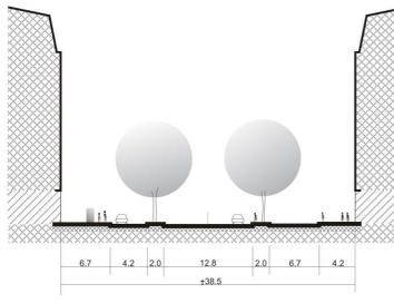
Figure 52 - Cross section Avenue Montaigne
