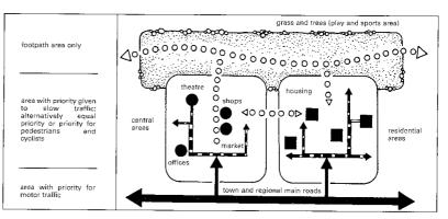
Figure 18 – Diagram representing the principle of cell and artery and the separation between pedestrian network and major traffic arterials (Source: Neufert, Third Edition, 2000)
