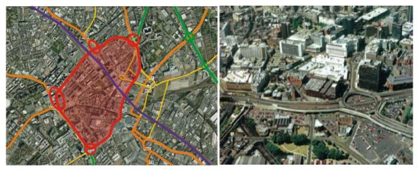
Figure 47 - Plan and photo of Birmingham's Concrete Collar Left - The Concrete Collar (figured in red) and the network of streets and motorways leading to the city's central area (in green – motorways, in orange – regional or local importance ways) – scheme O. Stepan Right – The interchange via slip roads constructed between the Central Ring and one of the median roads conforming to Manzoni's - Source: Walk 21, R. Tolley
