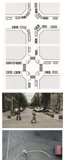
Figure 4 – Curb extensions used to reduce crossing distances and improve visibility for both pedestrians and drivers (Source: Calmar el trafico – Pasos para una nueva cultura de la movilidad -urbana, Gobierno de Espana, 2008)
