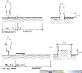
Figure 13 – Cycling paths physically separated from the roadway – Top: on the roadway by a raised curb; Bottom: between the roadway and the sidewalk (Sources: Manual de las vias ciclistas de Gipuzkoa, Diputacion Foral de Gipuzkoa, 2006 and www.eltis.org)
